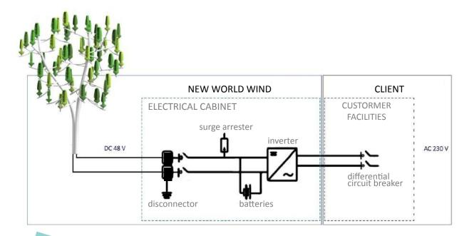
The Windtree is connected to the local grid through the NewWorldWind electrical cabinet. A dedicated space should be prepared for the cabinet, within a maximum distance of 20 meters. In addition to the WindTree and its electrical cabinet, NewWorldWind is also providing the electrical wires between the WindTree and the Cabinet.
